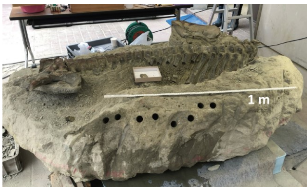
Fig. 2. Sandstone block containing the “Paleoparadoxiid Mizunami-Kamado specimen”, with eight holes where cores for magnetic measurements were sampled. Photo taken at the Mizunami Fossil Museum on December 17, 2022.
